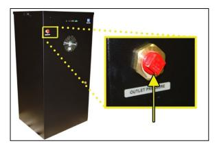
6.5.17 Connect the air supply line to the Outlet Pressure Port.
